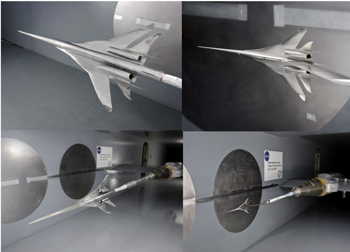
Figure 18 PM1 and BM1 Models Installed in the NASA Ames 9' x 7' Wind Tunnel During the Low-Boom Validation Test
