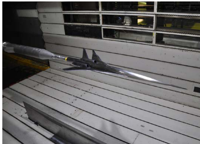
Figure 22 PM1 Model with the 14 inch Pressure Rail in the NASA Ames 11' Wind Tunnel
