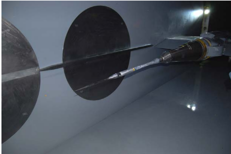
Figure 17 Boeing 2" Pressure Measurement Rail Installed in the NASA Ames 9' x 7' Wind Tunnel with the Boeing Body-of-Revolution
