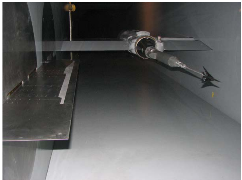
Figure 15 14" Pressure Measurement Rail Installed in the NASA Ames 9' x 7' wind tunnel with NASA LBWT Model
